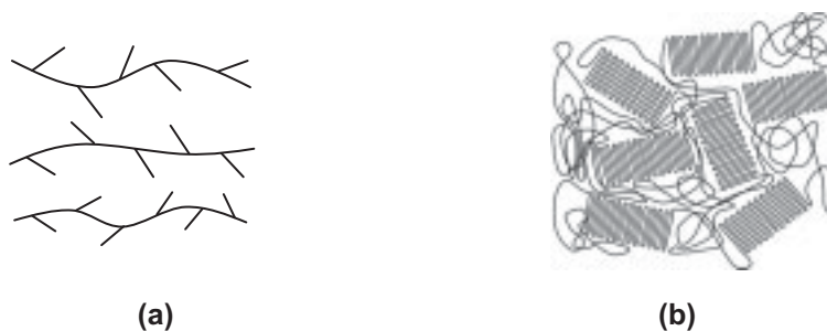
Figure 2.4 Schematic chain structures of (a) isotactic (upper), syndiotactic (middle), atactic (lower) molecules and (b) a crystalline polymer [37].
