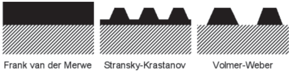
Figure 1: Different thin film growth modes as described in the text.
