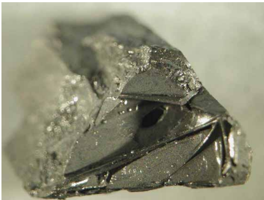
Figure 3.5: Single crystals of \text{YbFe}_2\text{Ge}_2 embedded in polycrystalline material.
