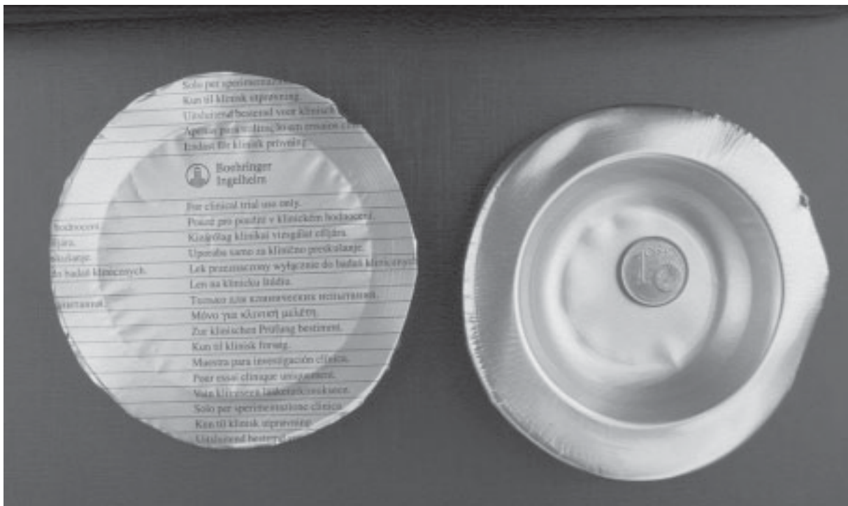
Figure 2.4 Large volume blister sealed (left) and opened (right, 1 €-cent for size comparison), prepared by the special device
