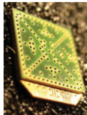
Fig. 5.12 (a): Test flip-chip integration of the chip onto the lower substrate stack. The chip is fed by the CPW line.
