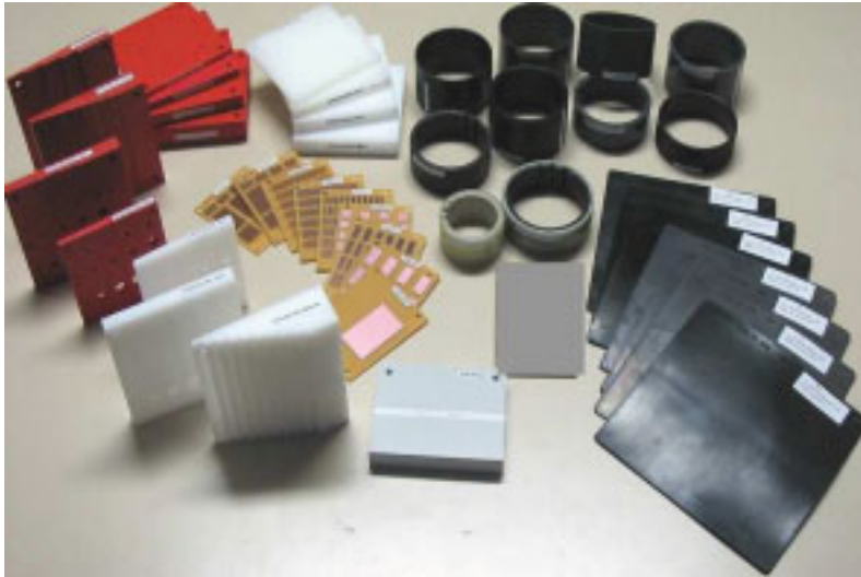
Figure 9.1: Test samples for THz non-destructive testing provided by BAM
