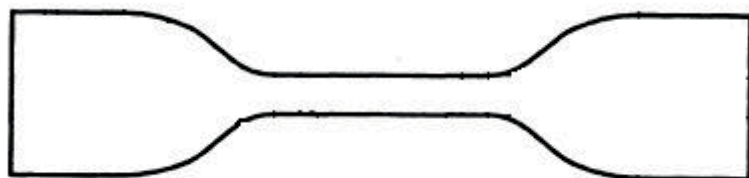
Figure 66: Test specimen type 5 according to DIN EN ISO 527-3.
