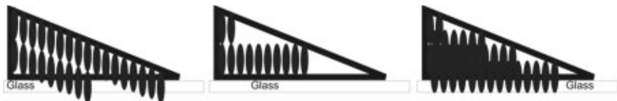
Figure 3.8 Schematic illustrations of different slicing strategies on the example of the microprism (side view).
