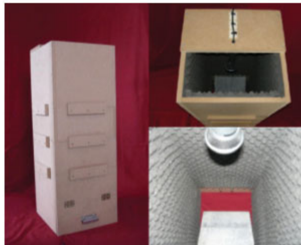
Figure 2 Complete Equipment and the installation of microphone and impact plate
