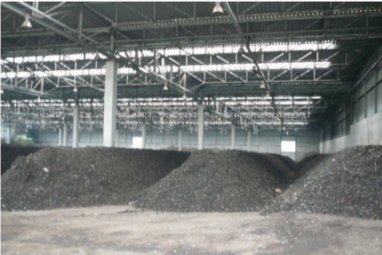
Figure 1: Maturation MBT Cröbern after changing to windrows
