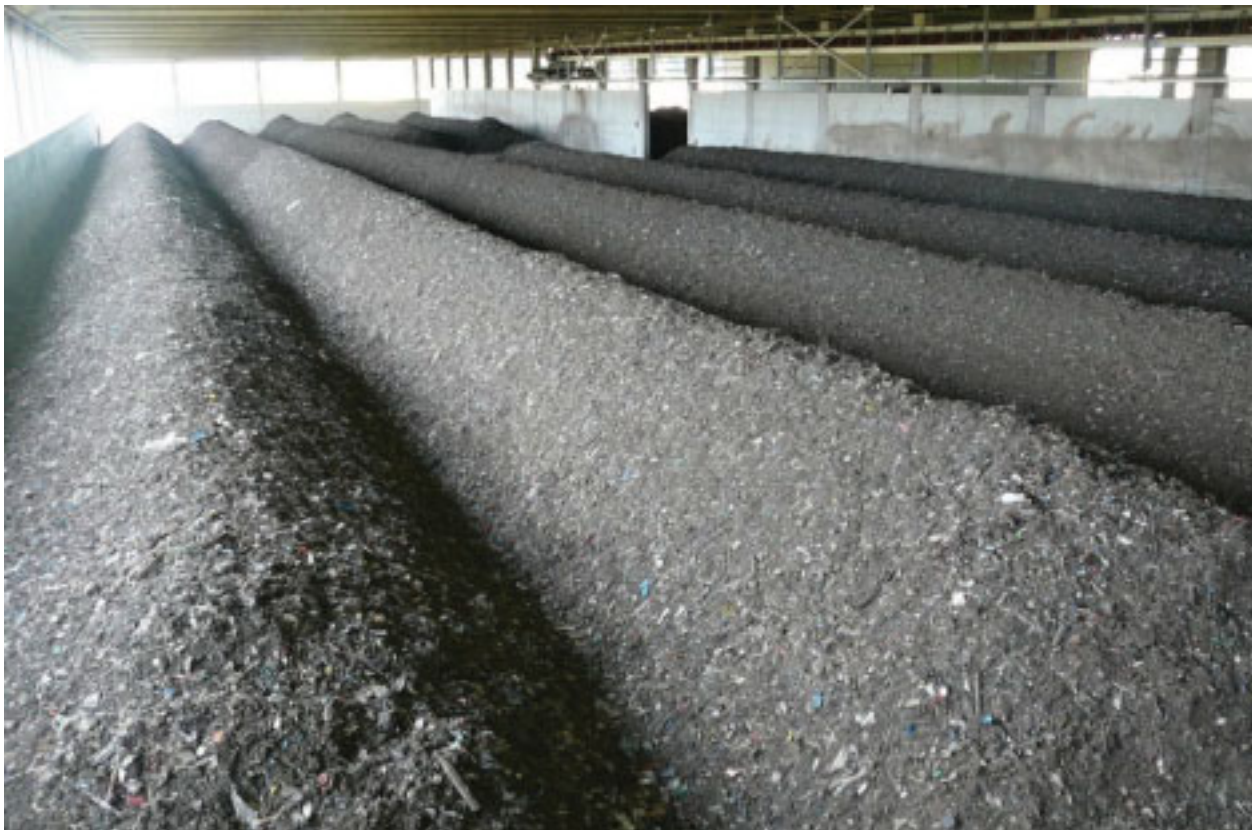
Figure 2: Maturation MBT Rosenow after reorganisation towards windrows
