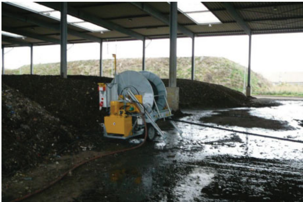
Figure 3: Maturation MBT Schwanebeck, irrigation unit
