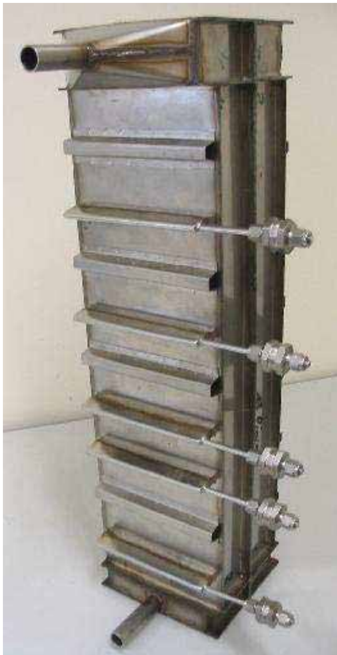
Figure F.6: Photo of the 10-kW Folded-Sheet Reformer for SRM. Notice that the 5 side-feed injection ports are provided with particle filters, avoiding the intrusion of solid particles to the gas distributor.
