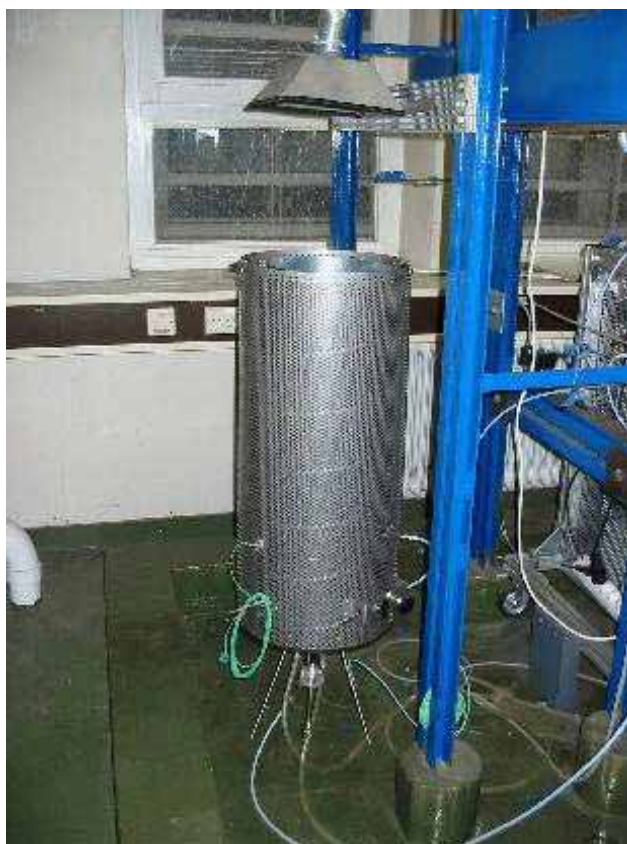
Figure F.7: Top: 10-kW Folded-Sheet Reformer installed in the experimental set-up. Bottom: Off-gas flame burner.
