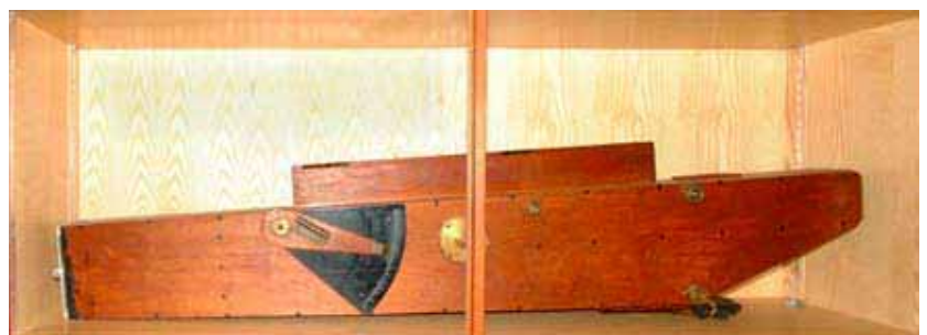
Fig. 8: One of the first Dobson spectrometers. Although emerging technologies have since allowed the development of a multitude of alternative ozone remote sensing methods, modern-day versions of the Dobson spectrometers still constitute the pillars of worldwide ground-based ozone monitoring networks. (Credit: University of Oxford, Atmospheric, Oceanic and Planetary Physics Dept.)
