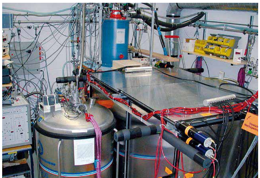
Fig. 5: The cryogenic ORPHEUS detector in the underground laboratory at Bern University has been used in the search for WIMPs. Due to their very weak interactions, the detection of WIMPs is extremely difficult and has not yet been achieved. See also Spatium-7: In Search of Dark Matter in the Universe.
