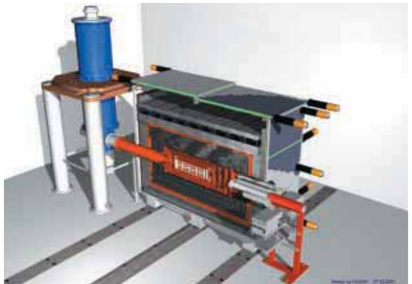
Figure 12 Cross sectional view of the ORPHEUS dark matter detector. The detector is horizontally connected via a side axis with a dilution refrigerator, which cools it down to a temperature of -273\text{ }^{\circ}\text{C} . It is surrounded by shielding material and scintillation counters to protect against background from particles other than WIMPs.
