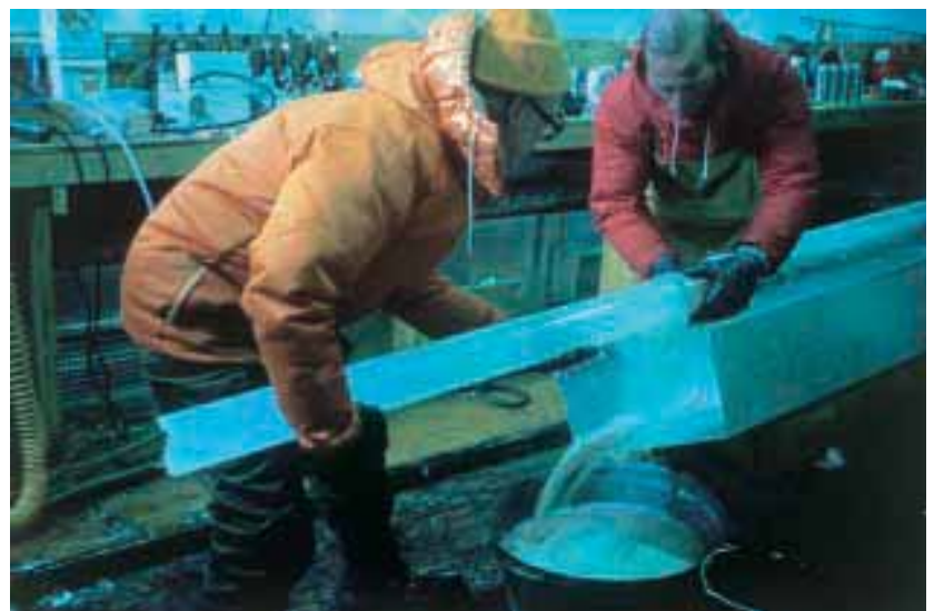
Figure 8 Deep-drilling (2,000 to 3,000 metres) is performed underground and takes about 2 to 3 years (Summer seasons). The drill is lowered into the borehole, drills a core of about 2,5 m length and is then brought up to the surface again. The picture shows how the ice-core is taken out of the drill. The liquid is used to prevent the borehole from closing.
