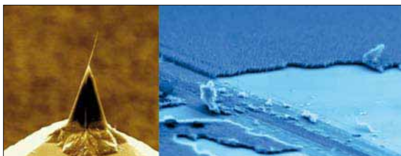
Figure 12: Glimpses into the nanoworld. On the left side, a carbon nanotube is depicted. Its thickness is a mere 10 atoms. The image to the right shows the structure of a carpet made up of such nanotubes.
