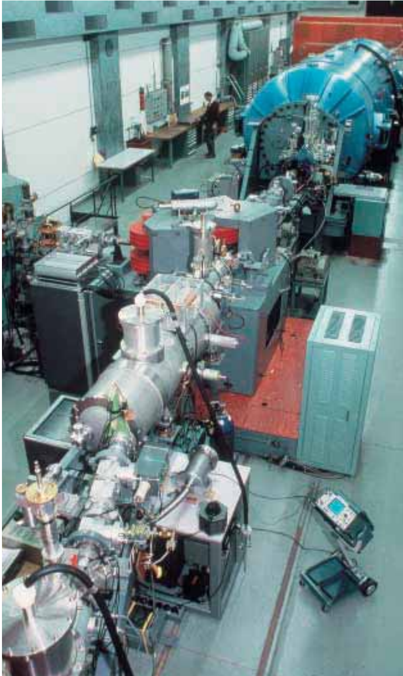
Figure 10 View of the accelerator mass spectrometer of ETH/PSI, which is used to measure the ^{10}\text{Be} concentration in ice. The central part of this instrument is the tandem accelerator (blue tank in upper right corner), which accelerates the Beryllium ions to very high energies (20 MeV). This is necessary to analyse ice samples of 1 kg containing as few as 10 million ^{10}\text{Be} atoms.
