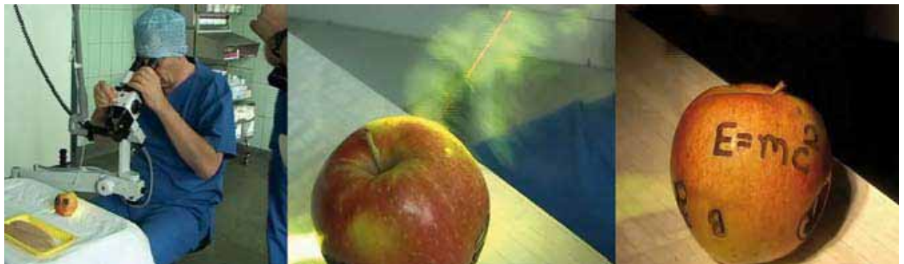
Figure 10: Einstein in the operating theatre. The coherent light of lasers finds an overwhelming variety of applications today. This sequence shows a surgeon demonstrating a carbon dioxide laser writing Einstein's famous formula on the skin of an apple.
