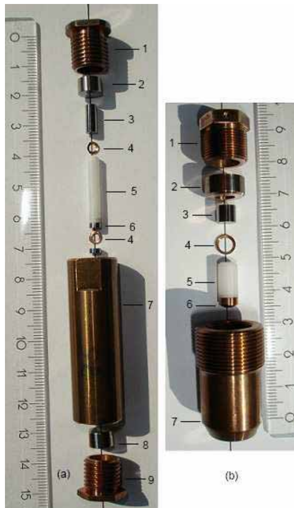
Figure 2.2: Piston-cylinder type pressure cells used for specific-heat measurements at low temperatures. Left photo (a): double-layer pressure cell (type II - Ni-Cr-Al inner layer, CuBe outer jacket); right photo (b): mono-layer pressure cell (type I - CuBe). The different components of the cells are indicated by numbers from 1 to 9. 1: locking nut (CuBe); 2: blocking disc ( a - tungsten carbide (WC), b - CuBe); 3: piston (WC); 4: sealing ring (CuBe); 5: POM capsule (sample space); 6: plug ( a - WC, b - CuBe); 7: main body of the pressure cell; 8: blocking disc ( a - Ni-Cr-Al); 9: locking nut (CuBe).
