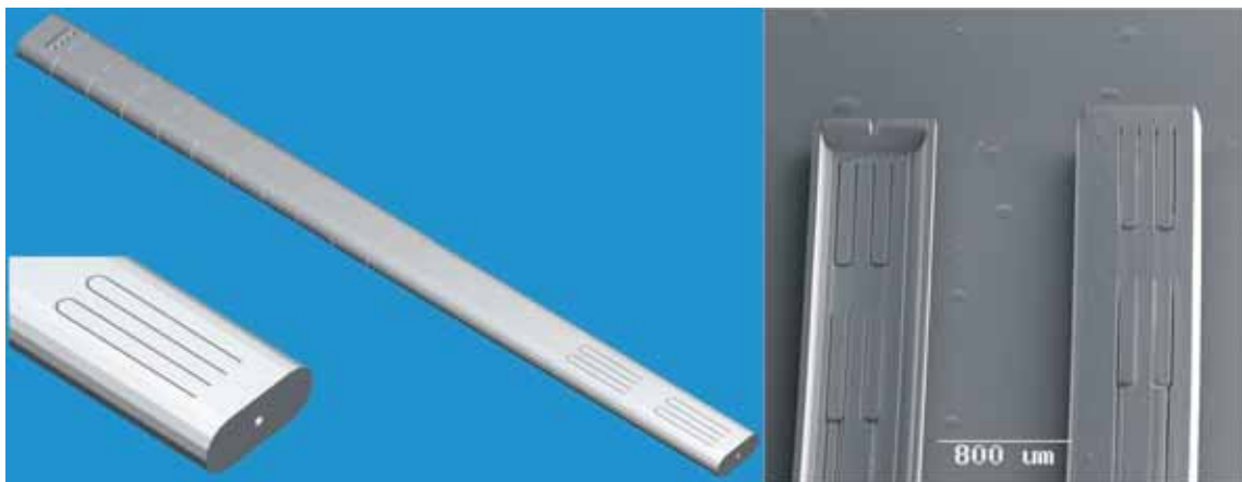
Figure 2.30.: The 10\text{ mm} long design for an ophthalmologic stent (left), a close-up of the stent exit with flap-valves (inlet), and a SEM image of the stent flap-valves of a 10\text{ mm} long stent fabricated by 2PP (right). The left fabricated stent was interrupted during fabrication to be able to look inside. For the use in ophthalmology, a stent with an outer diameter of less than 500\text{ }\mu\text{m} is needed. Furthermore, the valves and other design components of the stent are a novelty, which can not be fabricated using the standard stent cutting techniques. For this reason, this kind of novel stent is addressed in the 'Sonderforschungsbereich-Transregio 37' started in the middle of 2007 using 2PP fabrication technique.
