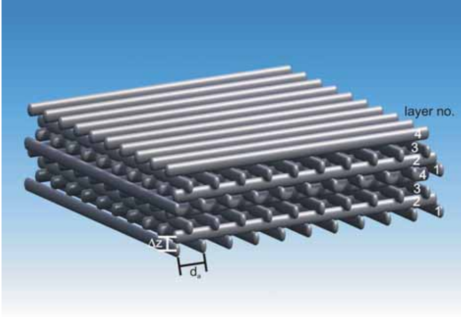
Figure 2.12.: The principal design of a woodpile photonic crystal showing the layer distance \Delta z , the lattice period d_a , and the layer number.
