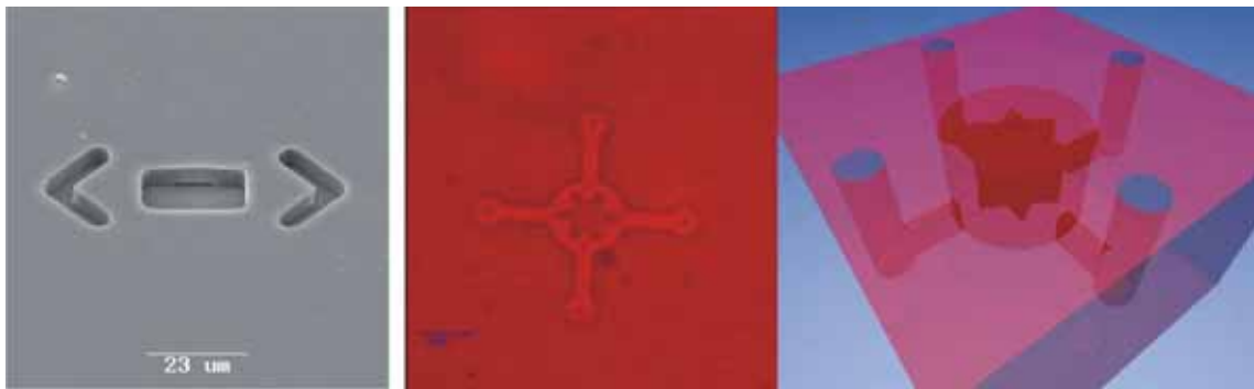
Figure 2.27.: A cut through a laser cavity for a dye laser (left), and a micro-fluidic mixer (right) fabricated using 2PP. The laser cavity with the fluid inlet seen at the top wall and the very good quality of the triangular mirror walls demonstrates the ability of 2PP in combining micro-fluidic and micro-optics. The micro-fluidic-mixer gives a first impression of the new possibilities and freedom to the design of micro-fluidic components enabled by the 3-dimensionality of 2PP. With the four channels connected through the polymer surface, while the middle chamber with the gearwheel has a cover layer of polymer and the gearwheel rotatable hung on an axis, the advantage of 3-dimensional structuring is demonstrated.
