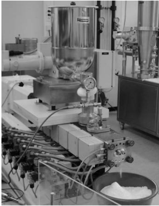
Fig. 6 Leistritz Micro GL 27 / 28 in the modified granulation setup
