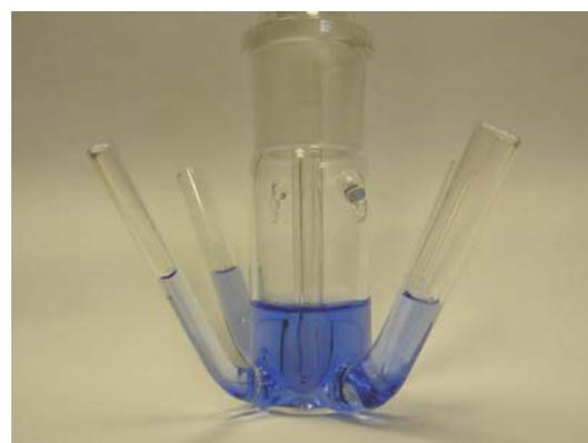
**Figure 3.** Picture of the reaction unit.
