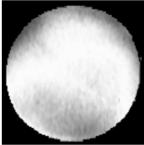
Fig. 5.3: Variations of the EW of the main transmission peak across the aperture of the TNF, tuned at 390 nm. The grayscale is defined as follows: black corresponds to 0 and white to the EW of an ideal TNF given by (5.3). Simulation based on the thickness maps of the individual etalons, provided by the manufacturer.
