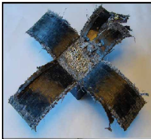
Figure 6.14: Crush pattern of foam-filled composite crash box
