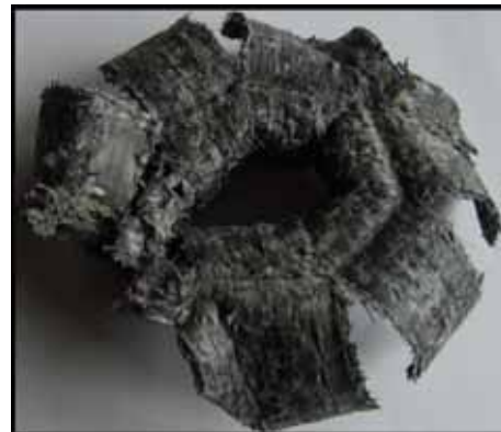
Figure 6.2: Crush pattern of square tube S-67 (left) and hexagonal tube S-75 (right)
