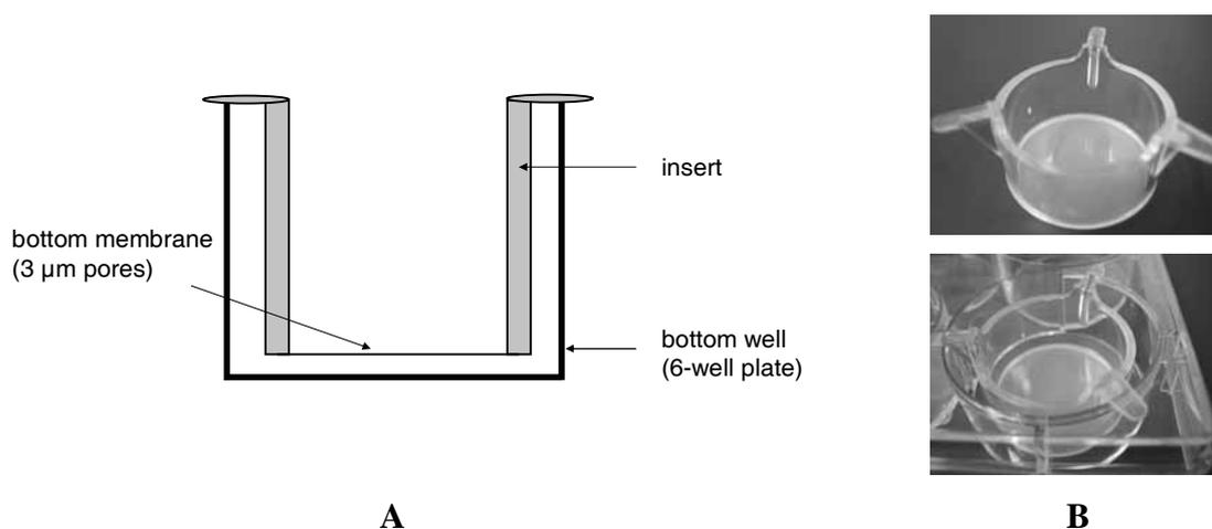
**Fig. 10** Membrane insert for a 6 – well plate used for the construction of the cornea equivalents. **A** = schematic illustration of a 6-well with the insert, **B** = pictures of the insert.
