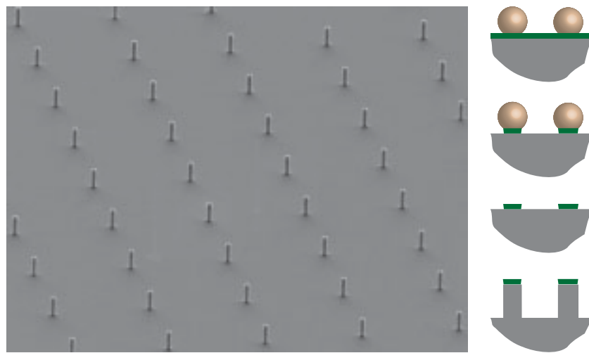
Figure 5.51: Silicon rods created via sparse colloidal lithography with 500-nm PS beads. The beads' footprints were transferred into an oxide layer via RIE, and the hard mask was transferred into the bulk Silicon via DRIE.
