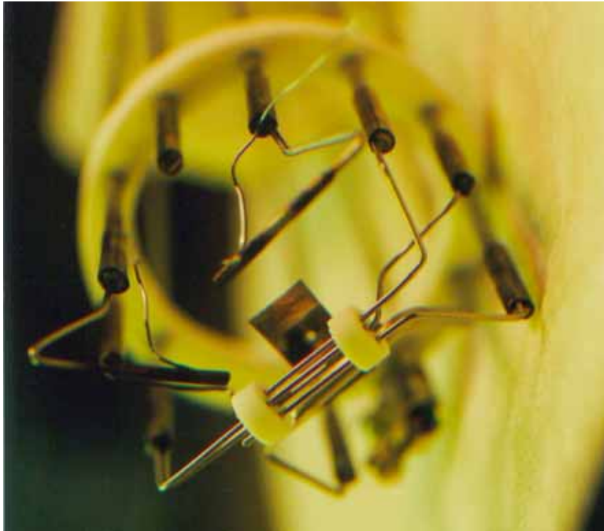
Figure 3.2: Photo of the linear trap before final assembly into the vacuum apparatus. The ovens are not aligned yet.
