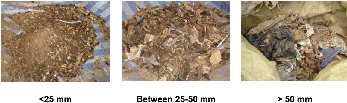
Figure 6 Fractional distribution of waste samples after trommel separation
