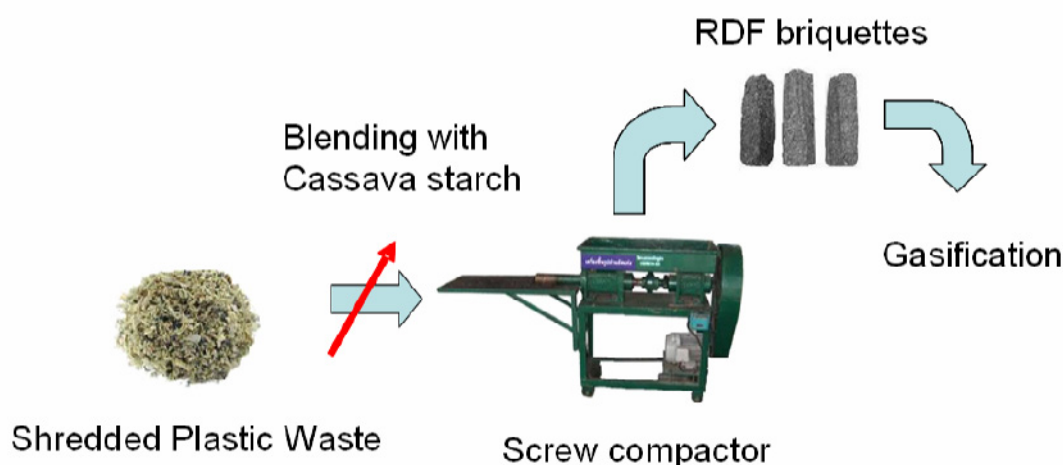
Figure 8 Steps involved in the production of RDF briquettes
