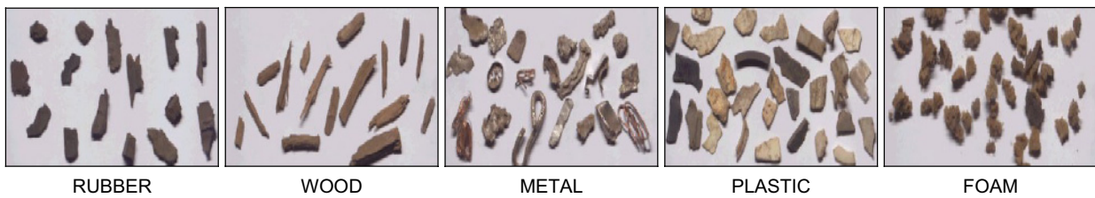
Figure 6 Examples of fluff samples belonging to five different classes of materials, utilized to perform the spectral analyses.
