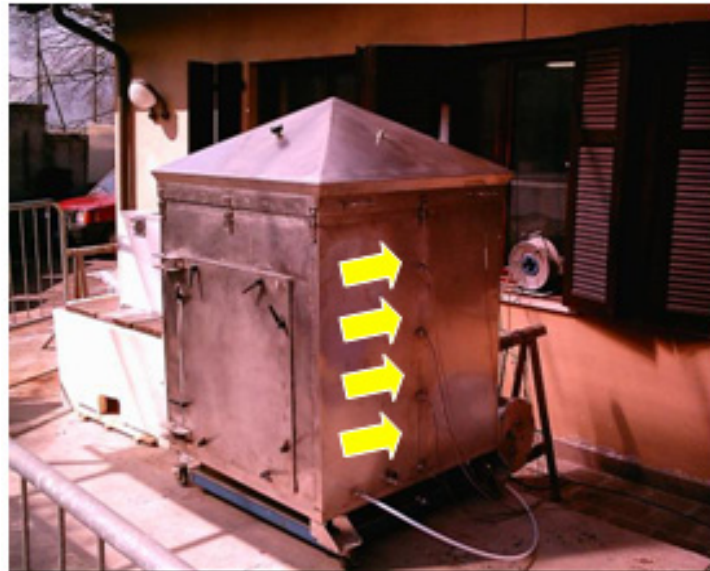
Figure 2 Frontal view of the biological reactor and position of the temperatures probes
