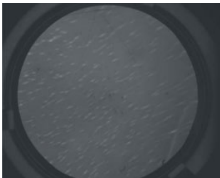
Figure 5.7. LEEM image of the Pt/SnO 2 surface before and after electron beam bombardment.
