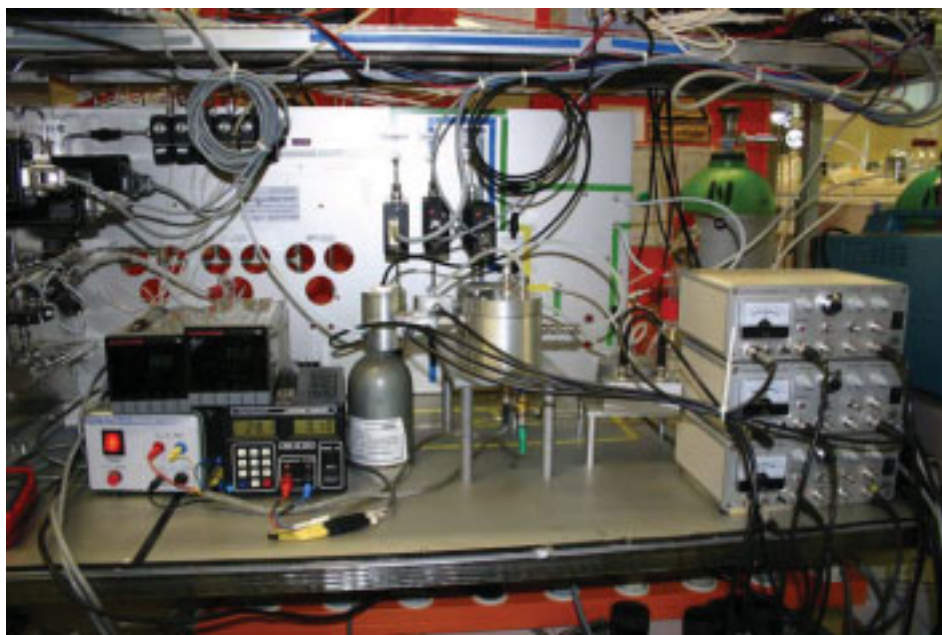
Figure 3.9. The Kelvin Probe-measurement station with three Kelvin Probe chambers and different operating temperature.
