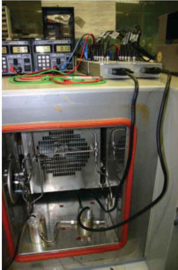
Figure 3.10. The FET measurement station. The sensor chamber is put in the climatic chamber. Two same or different sensors with ten transistors can be characterized.
