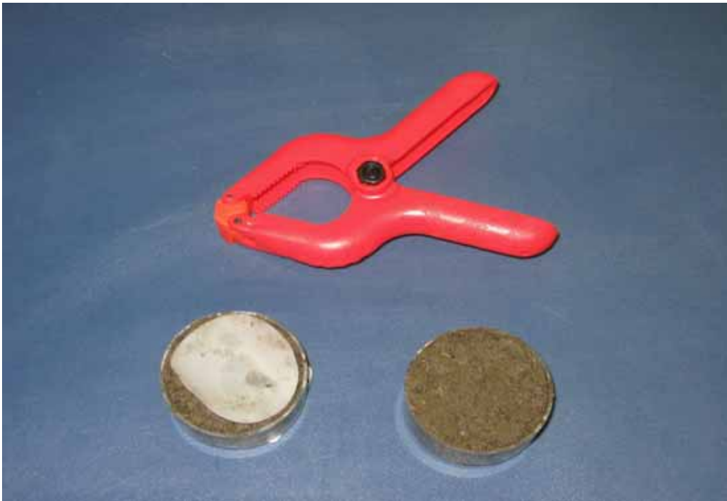
Figure 4. 1 “Sandwich” compositions: caps with soil, circular strip of ion exchange membrane, and clamp.
