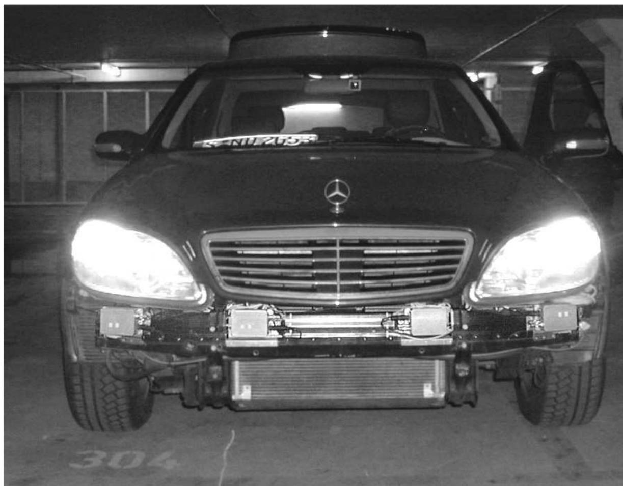
Figure 12.1: Passenger car equipped with a radar network prototype.
