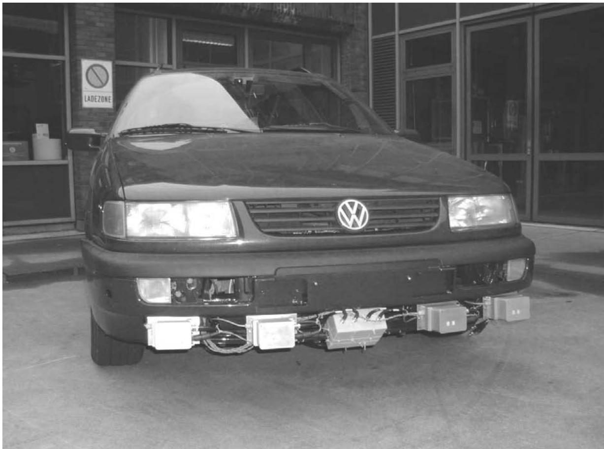
Figure 9.2: Experimental car equipped with the radar network
