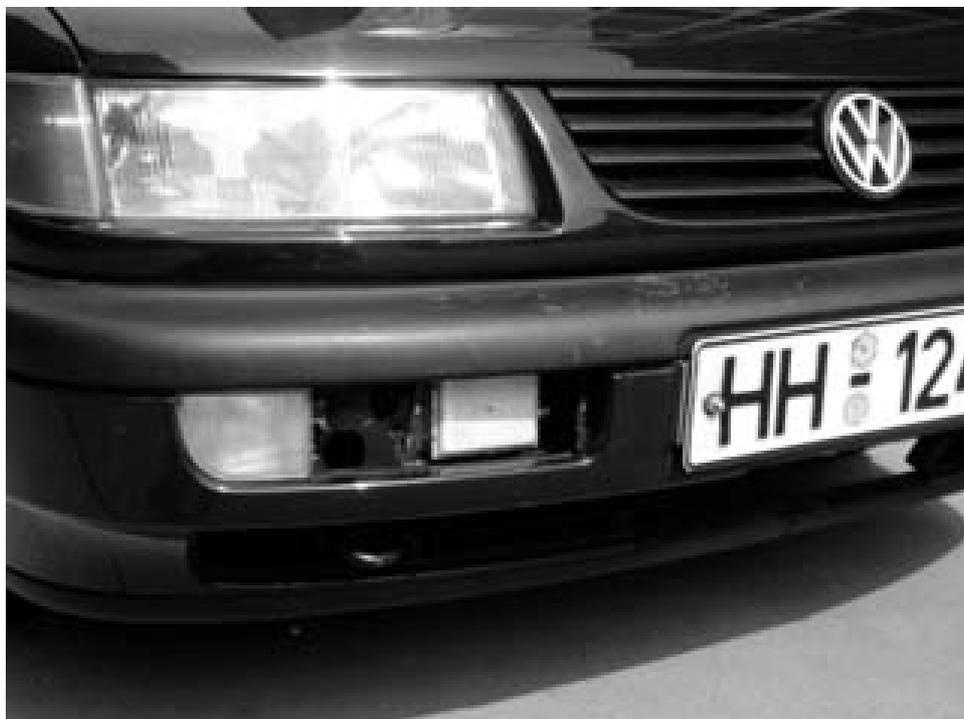
Figure 4.2: Detailed view of one UMR sensor in the front bumper
