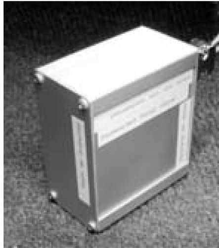
Figure 4.4: Turn rate sensor
