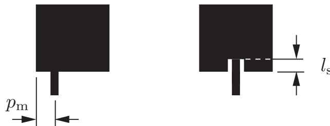
Fig. 4.13: Common techniques of impedance matching used for the feeding of a microstrip patch radiating element.
