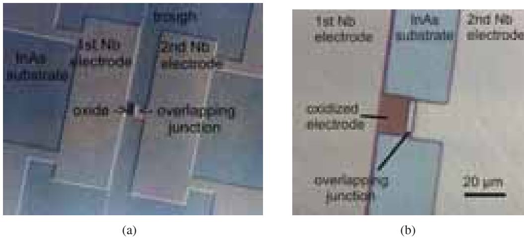
Figure 2.6: (a) Optical micrograph of an overlap junction. The oxide-covered part of the Nb electrode is marked by its dark color. The step in the substrate is the edge of the trough created by removing oxidized InAs. (b) Close-up of the junction area.
