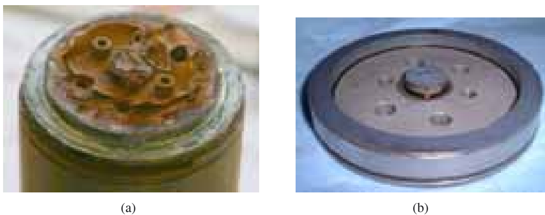
Figure A.4: (a) Corroded magnetron cathode after opening. Residues of the circular inner NdFeB permanent magnet and its capsule material are visible at the center. The outer ring magnet has disintegrated and could not be removed in one piece. (b) Same magnet assembly after cleaning and fitting with new magnets. The magnets are encapsulated with additional anti-corrosion varnish.
