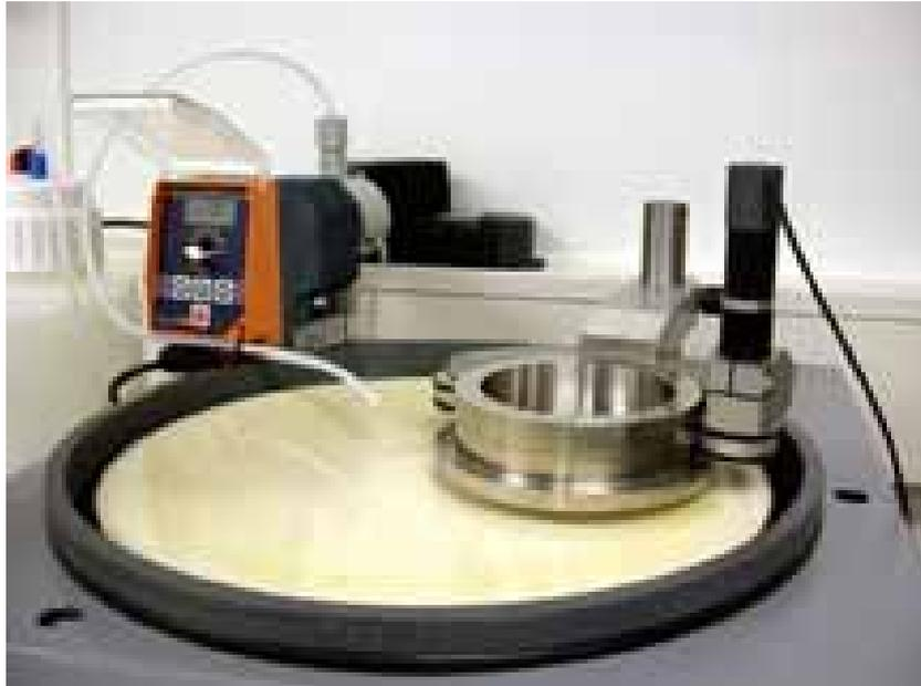
Figure 4.11: Close-up view of IBS PT 350 CMP polisher with monolithic polishing head (Fig. 4.12) during process. The electric motor powered roller for friction based forced rotation of the head is visible at the right end of the sweep arm. This setup was used for most of the results presented here.
