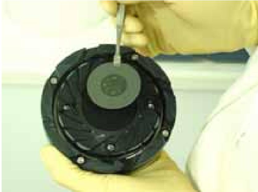
Figure 4.13: Placement of the quartz / silicon carrier wafer combination into the self-constructed wafer carrier attached to the underside of the IBS polishing head. The recess is lined with Rodel DF200 backing film. This latest version includes grooving of the contact surface in order to enhance slurry flow towards the wafer and is not yet qualified for processing.
