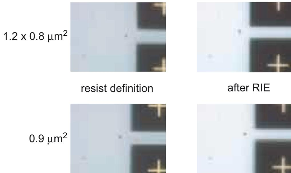
Figure 3.3: Initial e-beam definition and reactive-ion etch test with negative image ma-N2405 resist for real device features with junction areas depicted (light-microscopic image at  $1000\times$  magnification).
