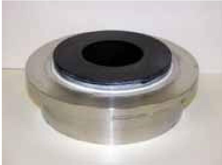
Figure 4.12: Monolithic polishing / head wafer carrier construction. The loading force is fixed by the weight of the stainless steel (V4A) body to an optimized value of 26 N. The black wafer carrier (100 mm diam.) is a precisely turned and lapped disk of mechanically and chemically resistant polyamide material (see Tab. 4.1) and bonded to the steel body (white silicon rubber sealing can be seen at the edge). The recess is  $1.27 \pm 0.01$  mm deep and lined with Rodel DF200™ backing film.
