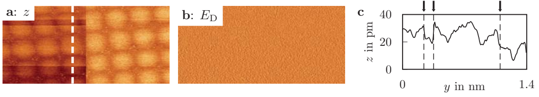
Figure 8.2: a (3 \times 1.4) \text{ nm}^2 MExFM image obtained using a Cr coated tip. The left side of the image represents raw data, while the right is flattened for better visualization. The image shows slight changes in z , while the magnetic contrast remains unchanged. b Simultaneously recorded dissipation showing no measurable contrast. c Line section along the white dashed line in a . Structural tip changes are indicated by black arrows.
