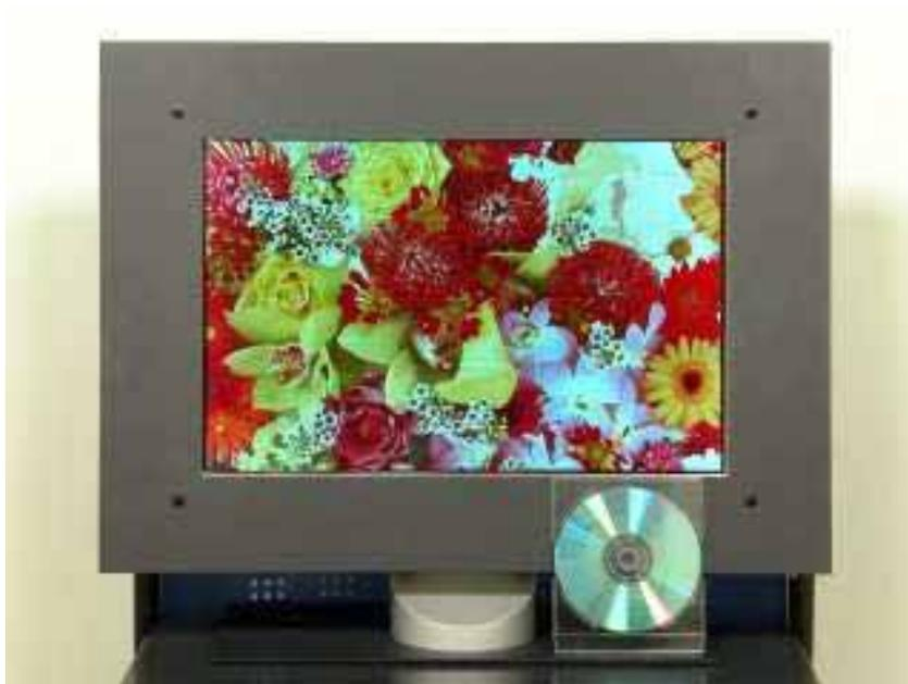
**Figure 1.2:** World's largest OLED display (20" diagonal) driven by a-Si TFTs developed in collaboration with IDTech, CMO and IBM Research [Tsumimura et al. 2003].
