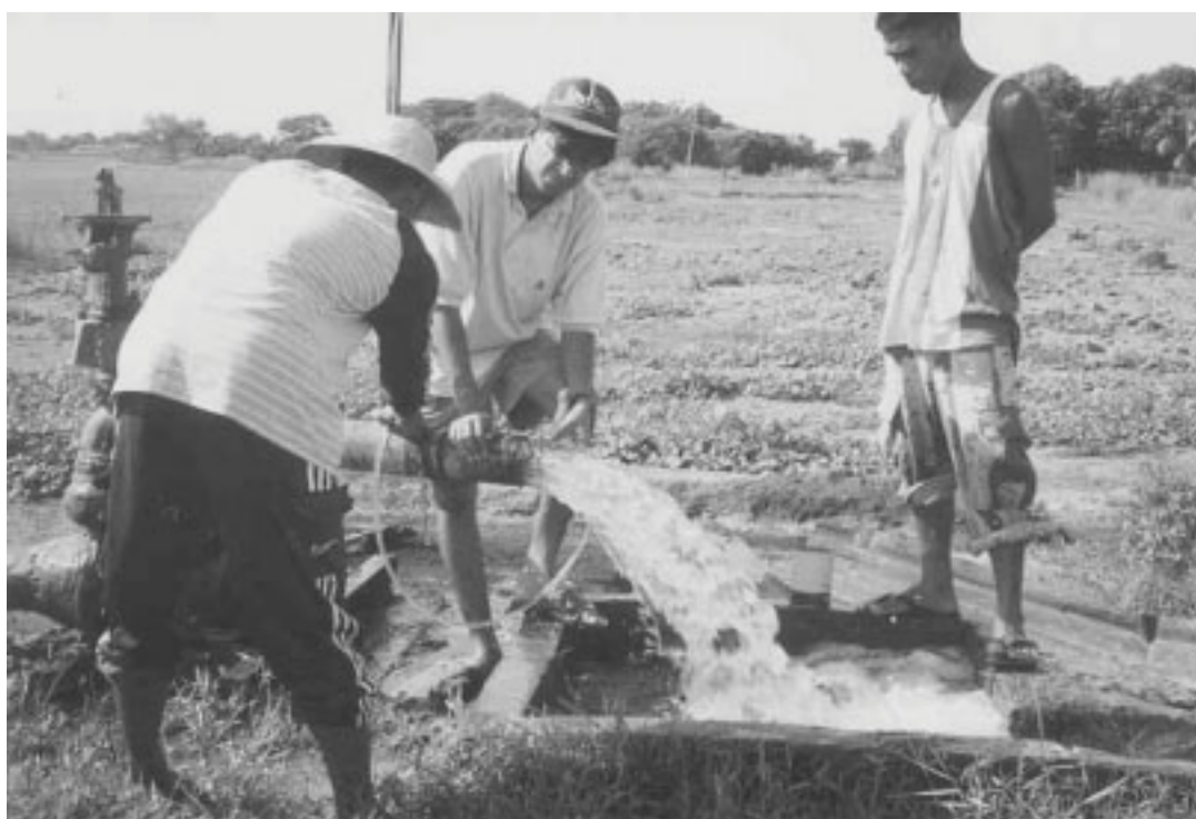
Figure 6. Pitot tube for calibration of the actual pump discharges.
