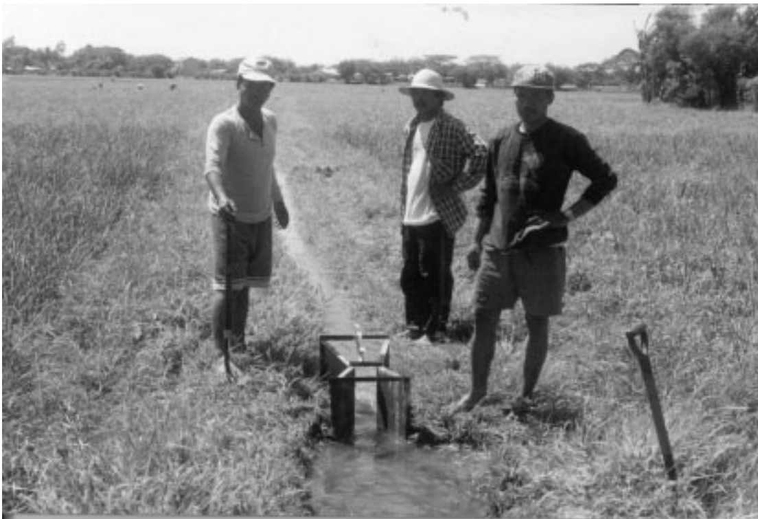
Figure 4 V-notch weirs for calibration of staff gauges along the small canals/creeks
