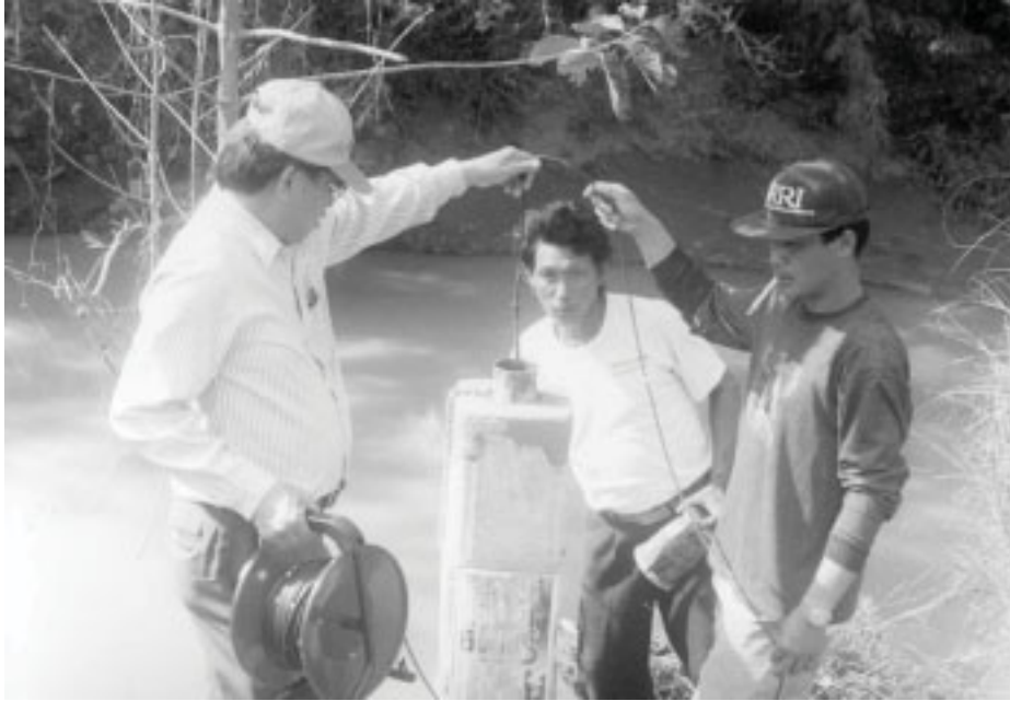
Figure 3.6: Experimental set-up for measuring groundwater level
