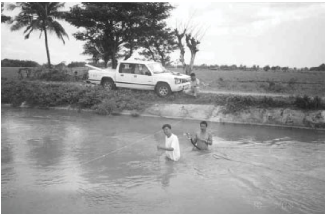
Figure 2. Staff gauge calibration using a current meter in the irrigation system
