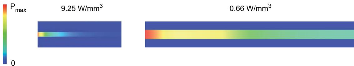
**Figure 2.18:** Heat load distribution in the  $ac$  plane for the 808 nm (left) and 888 nm (right) systems.
