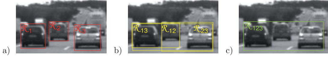
Figure 6.7: Example for region merging. In (a) three cars are detected (regions \mathcal{R}_1, \mathcal{R}_2, \mathcal{R}_3 ). These can be merged into three bounding rectangles containing two cars (b, regions \mathcal{R}_{13}, \mathcal{R}_{12}, \mathcal{R}_{23} ), and into one bounding rectangle containing three cars (c, region \mathcal{R}_{123} ). The combined regions found in (b) and (c) are then added to the original list of candidate regions from (a).
