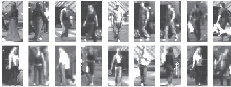
Figure 5.3: Positive pedestrian samples with a resolution of 20 \times 40 px manually selected from the video sequences acquired with the test-vehicle and supplemented with positive samples from the DaimlerChrysler Pedestrian Classification Benchmark Dataset.
