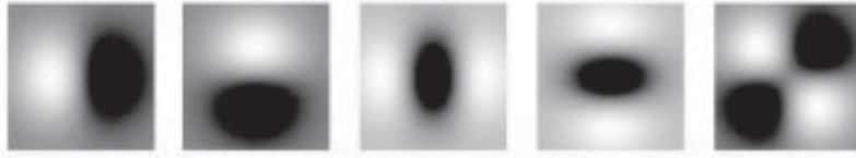
Figure 5.27: Five first and second order directional derivatives of Gaussian kernels used for feature space convolution. Source: Collomosse and Hall [119].
