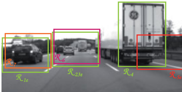
Figure 7.4: Candidate regions from Fig. 7.3 are extended. Note that \mathcal{R}_5 remains at its original size, since it is too large to be observed by high-resolution sensors.
