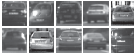
Figure 5.7: Positive car samples with a resolution of 32 \times 32 px manually selected from the video sequences acquired with the test-vehicle.
