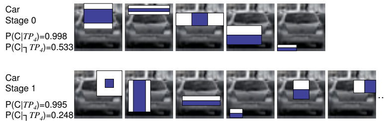
Figure 5.8: Haar-like features of stages 0 and 1 of the car classifier cascade with a minimum true positive rate of 0.997 shown in front of an example car image used for feature training. For each stage, the resulting rate of true positives P(C|TP_4) and false positives P(C|\neg TP_4) is given.
