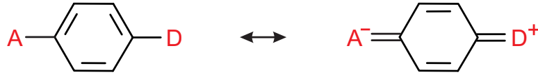
Figure 7.3: Ground state and low-lying charge-transfer excited state of a polar molecular unit. The structure possesses large values of the hyperpolarizability \beta (adapted from [138]).
