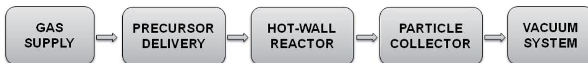
**Fig. 3.1.** Sequences of unit operations in a CVS setup
