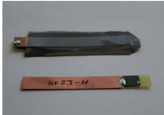
Figure 4.3: Photographs of NCD electrodes after contacting with silver paste (down) and after passivation with a Teflon-based adhesive tape (top)
