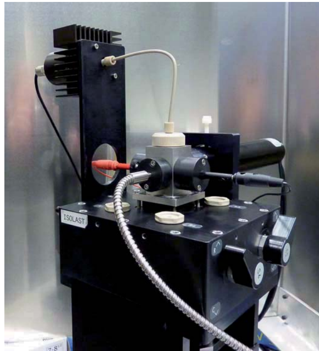
figure 2.2 Setup for simultaneous measurements in turbidity and conductivity mode. Observation head with optical fiber (silvery cable) and detector (photo cathode with secondary electron multiplier tube/PMT) in 180 ° angle. Perpendicular cable (red and black) to connect the electrodes at the flow cell with the detection unit
