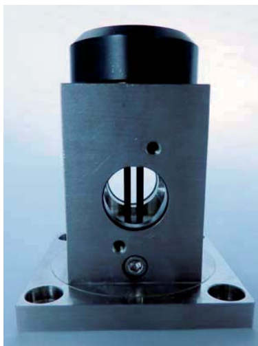
figure 2.1 Observation head of a SFM400/S stopped-flow device. Inside the head the standard measurement flow cell (fluorescence cuvette: FC-15) with an edge length of 1.5 mm and four transparent sides for measurements in transmission or fluorescence mode is visible. The mixture passes the head from the bottom to the top
