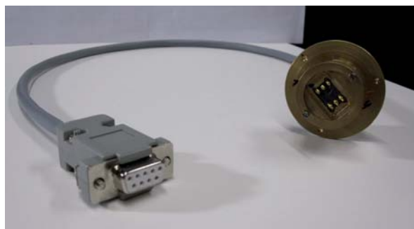
Figure 3.15: Custom sample holder for non-standardized samples.
