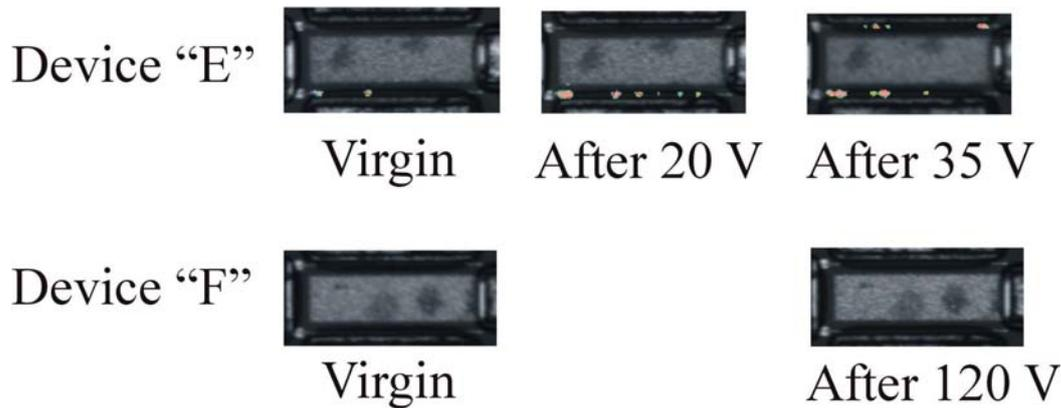
Figure 5.16 Superimposed images show evolution of EL spots at OFF-state ( $V_{GS} = 7$  V and  $V_{DS} = 10$  V) during step stressing. The measurements have been taken as indicated in Fig. 5.13. Note: EL intensity is not normalized.
