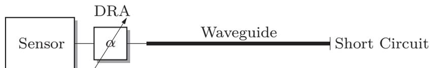
**Fig. 3.20:** Measurement setup for sensitivity tests.
