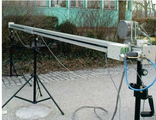
**Fig. 5.9:** Photograph of the overall setup for evaluating stripmap SAR at 77 GHz.
