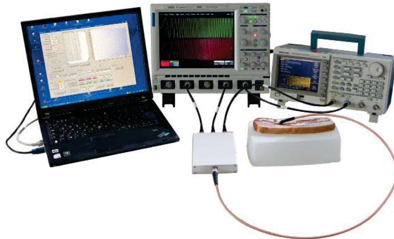
Figure 2.54: Photograph of the developed chirp signal measurement setup. A custom software running on a laptop computer controls the laboratory measurement devices and processes the sampled raw data.
