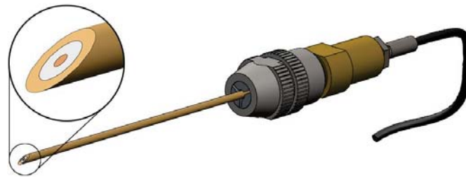
Figure 2.34: Prototype of a solid coaxial needle as constructed for the first experiments. The measurement signal is fed to the needle tip on the inner conductor. The outer wall of the needle serves as a grounded reference electrode which is isolated from the inner conductor.
