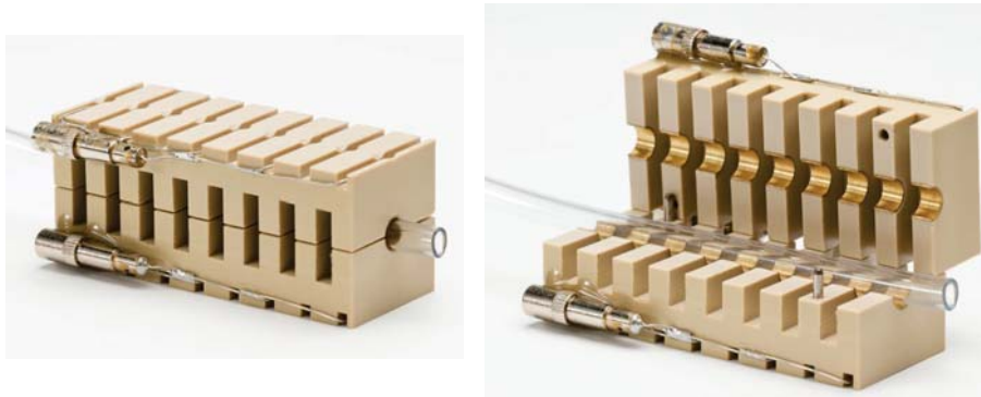
Figure 2.20: Prototype of a HCT sensor based on the concept with ring electrodes having a width of 5 mm and a distance of 3 mm to each other.
