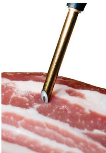
Figure 2.36: Photograph of a coaxial needle tip which is inserted into biological tissue during laboratory experiments.
