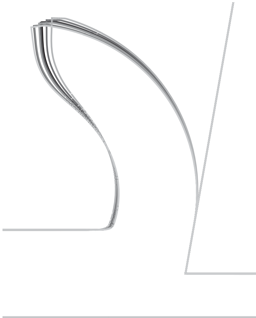
Figure 4.24: Overlay of chip shapes from adiabatic simulations at rake angle of +10^\circ using different Johnson-Cook parameter sets
