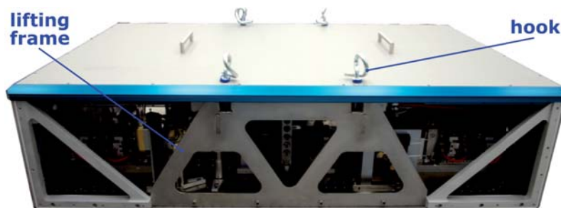
Figure 6.2: High power oscillator prior to shipment with installed lifting frame, top lid and hooks - the side is removed for illustrative purpose only.
