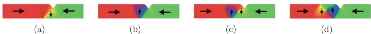
Figure 2.15: Models of transverse (a, b) and vortex-type (c, d) domain walls with clockwise (a, c) and counterclockwise (b, d) sense of rotation. Reprinted with permission from [Hay06b]. Copyright 2006 by the American Physical Society.
