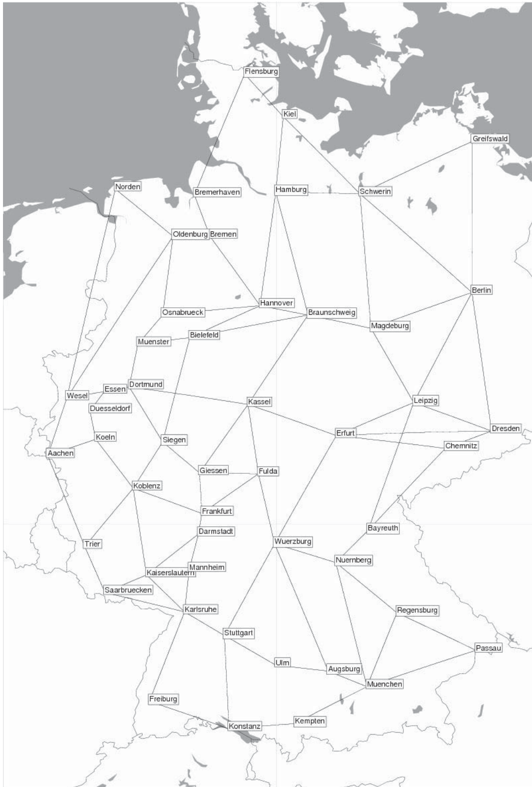
Figure 1.8: Example network design instance. The GERMANY50 instance and this picture are taken from SNDlib [130, 131], a public problem library for the design of survivable networks. This instances was originally provided to SNDlib by T-Systems International AG.
