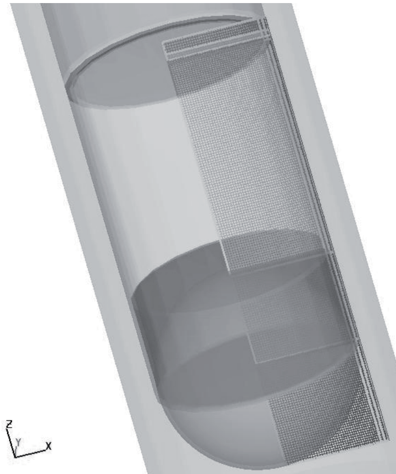
Figure 4-17. View of the dewar and the 2 dimensional cylindrical mesh.
