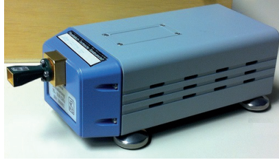
Figure 3.4 Frequency-multiplier chain (Radiometer Physics, FE-110, multiplication factor 6, output power \approx 10 dBm) with a W-band horn antenna (75-110 GHz).
