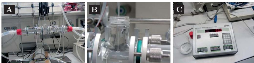
Figure 3.5: Dissolved oxygen measurement in hydrogels with microelectrodes. A: Section of the test site, B: Zoomed in on section of BTR with microneedle, C: micro-manipulator controller.
