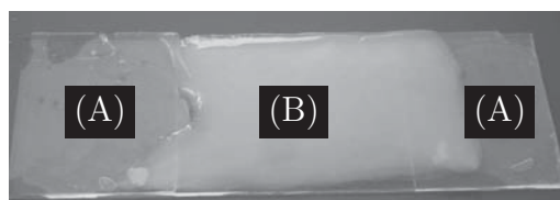
Figure 3.1: Object slide with in hydrogel immobilized cells: (A) Coverglasses glued to the object slide, (B) with hydrogel filled molding.
