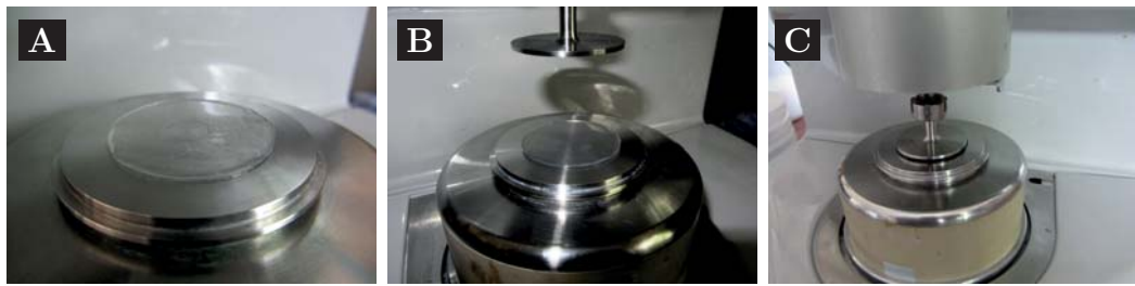
Figure 3.6: Hydrogel measurement with plate-plate. A: Hydrogel placed on bottom plate, B: Hydrogel between both plates, C: Hydrogel during measurement.
