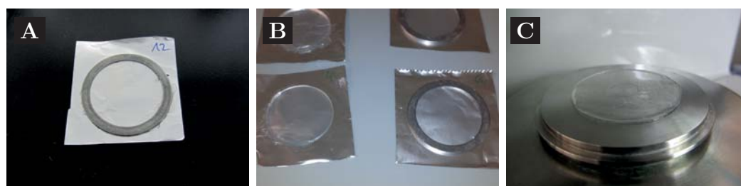
Figure 3.4: (A) Mold for the hydrogel, (B) hydrogel with and without mold, (C) hydrogel placed on the rheometer.
