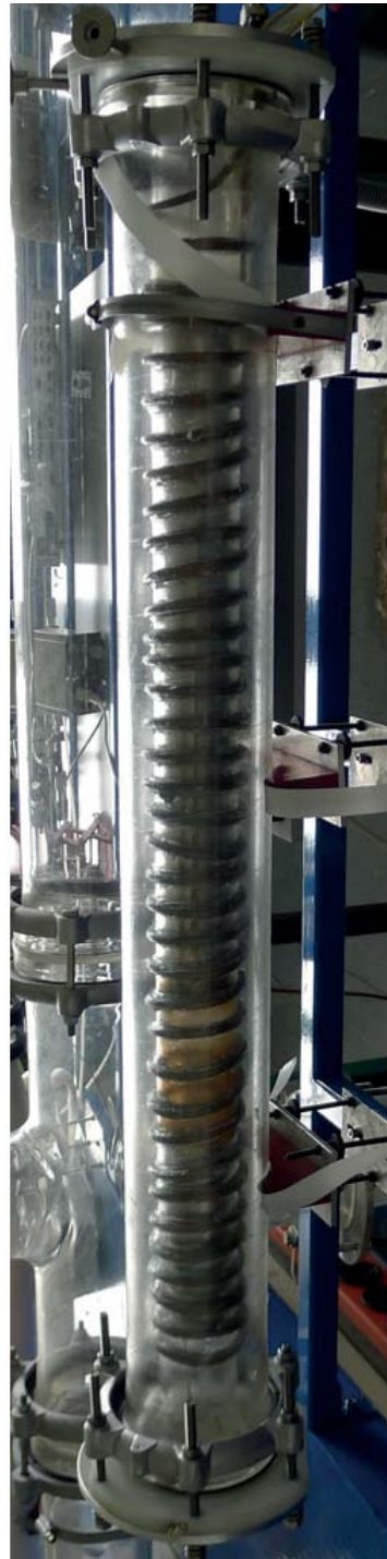
FIGURE 3.6: Old discharge cell used for the laboratory work described in Chapter 4. It is composed by two glass cells, one inside the other. The inner cell contains the electrodes and is surrounded by a copper solenoid used for cooling.
