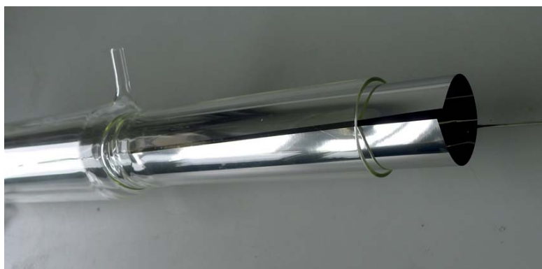
FIGURE 3.10: Example of a stainless steel electrode inside the new cell.
