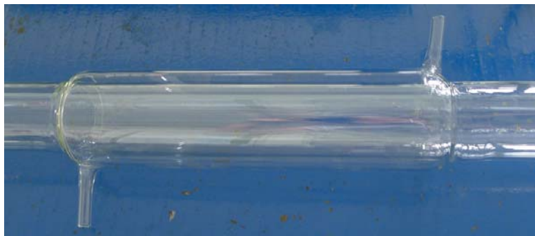
FIGURE 3.9: Jacket cell cooling system. A prototype of the new discharge cell made by the glass blower at the University of Cologne. It is composed by two layers. The outer layer is used for cooling the inner cell, where the electrodes are placed.
