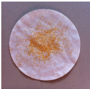
Figure 3-34: Standard corrosion test according to DIN 51 360 from pure water. Strong corrosion is observed on the filter surface.
