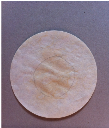
Figure 7-1: Corrosion test according to DIN 51 360 of DWME 2420 features an unchanged filter surface.
